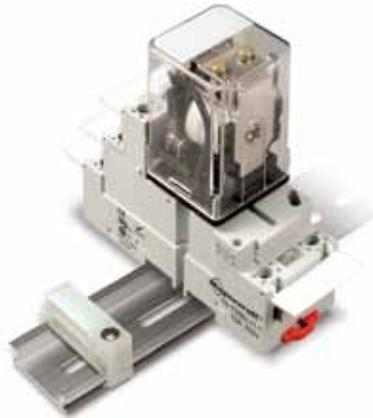
The 755 Magnetic Latching relay, with an 11 pin octal base, operates by using a pulsed input. A permanent magnet maintains the last position until a redirected second pulse moves the contacts back to the original state.
